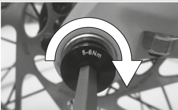
Figure 23: Tightening the securing screw
