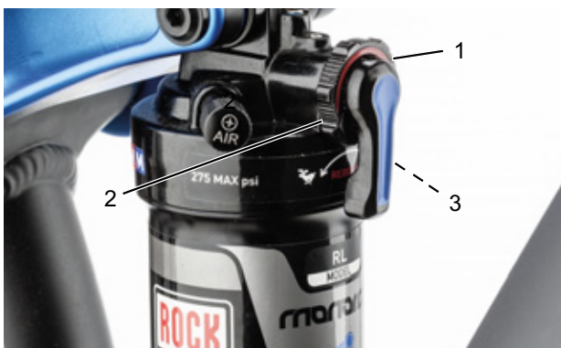
Figure 67: Setting the rebound damper strength on the rear frame damper setting wheel (1)
