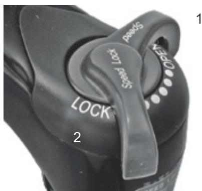
Figure 64: Suntour compression adjuster with the OPEN (1) and LOCK (2) positions
