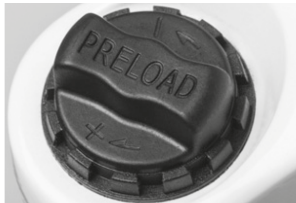
Figure 52: Negative deflection setting wheel on the suspension fork crown
