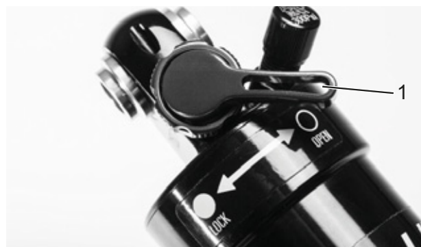
Figure 65: Suntour compression adjuster open (1)
