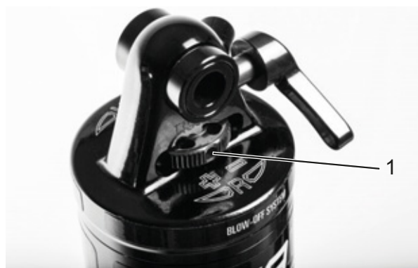
Figure 55: Suntour rebound adjuster wheel (1) on the rear frame damper
